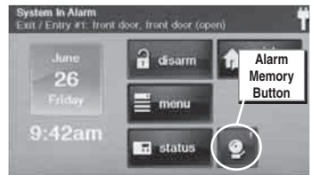
Security Screen with Alarm Memory Button
